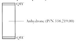
Adsorption trap (P/N 281.131.00) Adsorption trap o-ring (set of 2) (P/N 290.136.03)
