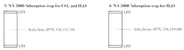
NA 2000 Adsorption trap (empty) (P/N 281.130.60) O-ring for NA 2000 Adsorption trap (set of 2) (P/N 290.100.82)
