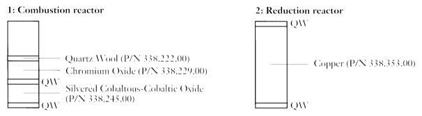
Combustion/Reduction reactor (set of 2) (P/N 468.200.00) Combustion/Reduction o-ring (set of 10) (P/N 290.329.10)
