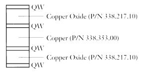
Combustion/Reduction reactor (set of 2) (P/N 468.200.00) Combustion/Reduction o-ring (set of 10) (P/N 290.329.10)
