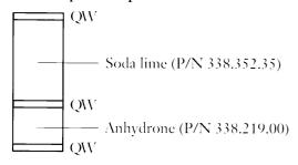
Adsorption trap (P/N 281.131.00) Adsorption trap o-ring (P/N 290.136.03)
