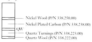
Pyrolysis reactor (set of 2) (P/N 468.200.00) Pyrolysis o-ring (set of 10) (P/N 290.329.10)
