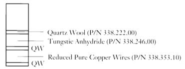
Combustion/Reduction reactor (set of 2) R (P/N 468.200.00) Combustion/Reduction o-ring (set of 10) (P/N 290.329.10)
