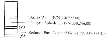
Combustion/Reduction reactor (set of 2) (P/N 468.200.00) Combustion/Reduction o-ring (set of 10) (P/N 290.329.10)
