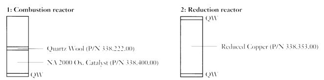
Pre-packed Combustion reactor (P/N 468.006.60)
