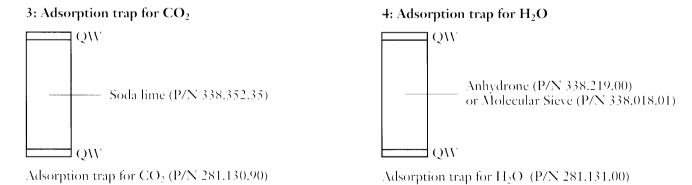
Adsorption trap o-ring (set of 2) (P/N 290.136.03)
