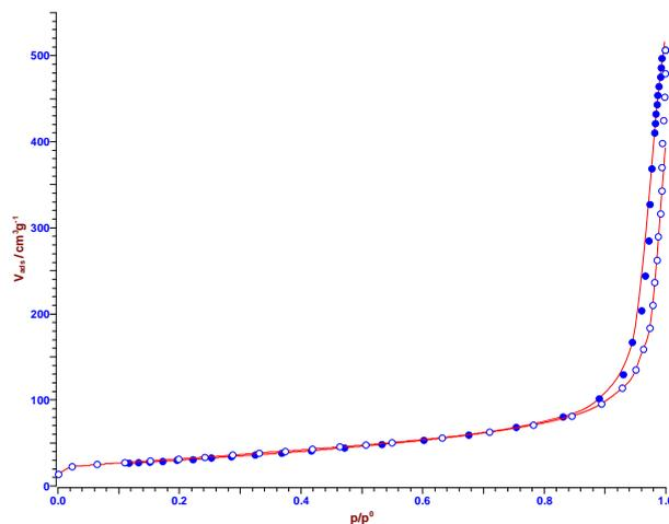
Figure 3 – Adsorption isotherm on carbon black
