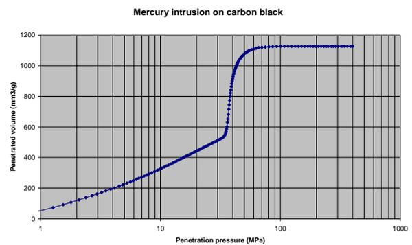
Figure 1 – Mercury intrusion curve on carbon black nano-powder
