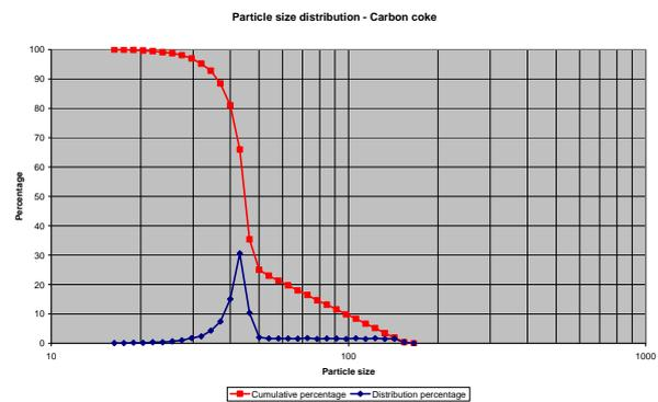
Figure 2 – Particle size distribution plot for carbon black nano-powder using  $k_p=3$ , contact angle= $124^\circ$ , hg surface tension= $480$  dyne/cm, real density= $2$  g/cc
