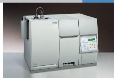
The most common measurements for catalysts characterization as TPD, TPR, TPO and pulse chemisorption are now easy to be performed and completely unattended by the new TPDRO 1100. The detector is a TCD type, which makes this instrument extremely sensitive, providing the solution for a large range of linearity. The TPDRO can automatically perform sample pretreatment simultaneously to the analysis on two separate and independent ports.
