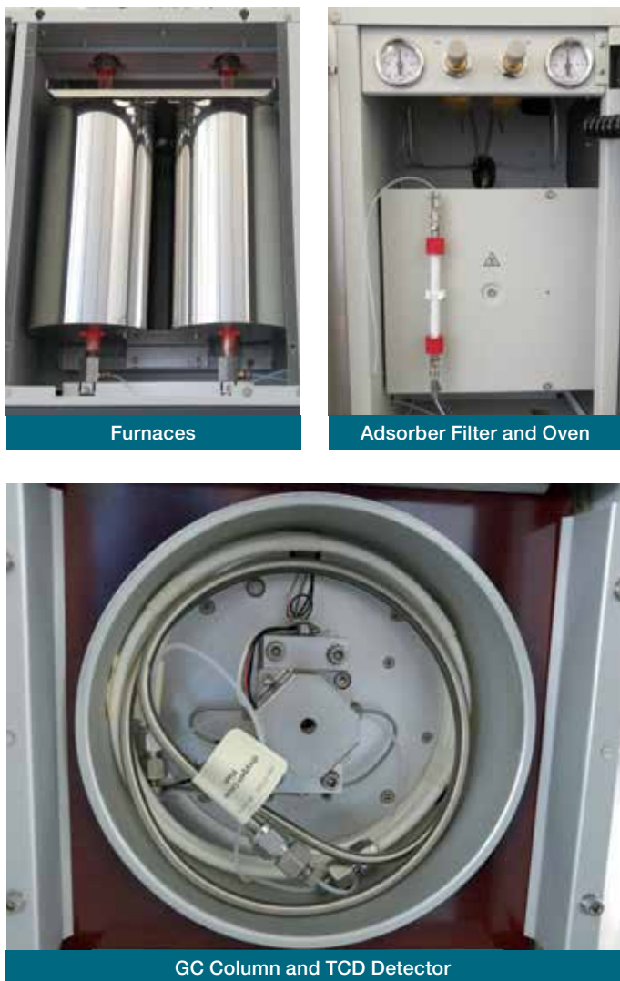
Figure 4. FlashSmart CHNS and oxygen internal circuits.
